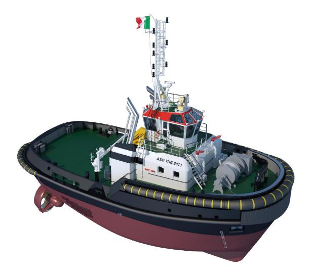
High performance towing and escort tug designed for efficient ship maneuvering and assistance to very large ships. Developed to offer truly superior ship-handling and seakeeping performances, this unit is able to docking and escorting ships in more extreme conditions than ordinary vessels.
